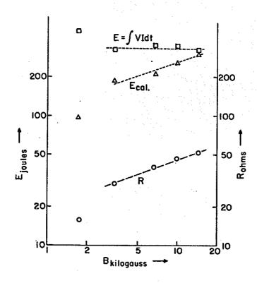
Figure 4 Diode impedance, R, Energy received by calorimeter, Ecal and energy computed from voltage and current traces E, vs. applied magnetic field, B.
