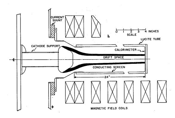
Figure 1 Experimental Schematic (Darkened area represents electron beam flow).
